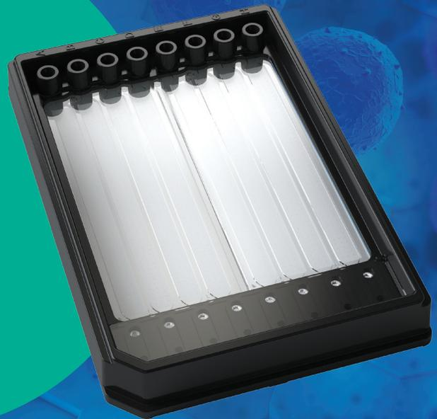
With the new flexible cartridge design, users may run up to eight tests on the same cartridge. Not only does the 8-lane cartridge allow higher throughput, it also introduces partial-use applications.
