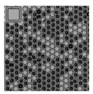
Significant cell loss after second bead wash: Images after cell loading
