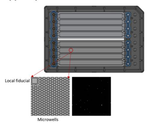
2. Note the location of the image within the microwell array by recording the location of the fiducial (post), in order to image the cartridge at the same location for Cell Load, second Bead Wash, and Bead Retrieval steps
