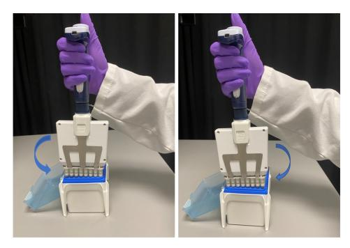
Tilt/Rock the pipette toward either side of the pipette tips (placed in a column as shown above) a couple of times to ensure a proper fit.
