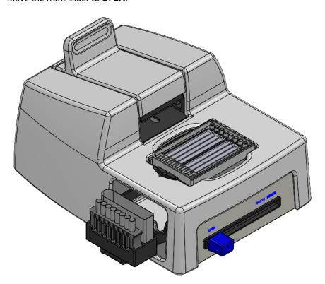
3. Remove the cap of a waste collection container. Insert both the waste collection container and the cluster tubes for bead retrieval into the appropriate slots in the drawer. When using partial lanes, use the corresponding number of tubes for sample retrieval.
