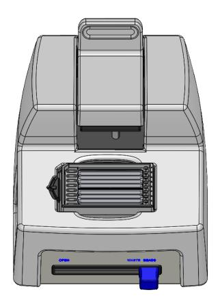
3. Gently pull the top **RETRIEVAL** slider onto the BD Rhapsody™ 8-Lane Cartridge (ACTIVE). Make sure that the Retrieval magnet is in contact with the BD Rhapsody™ 8-Lane Cartridge.
