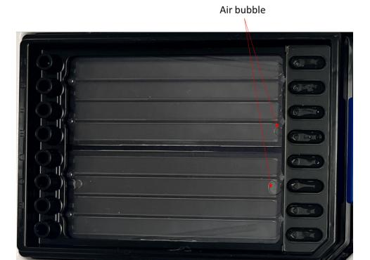
Air bubbles in a cartridge are rare. If there is an air bubble, proceed with the experiment. Follow the user guide to prevent introduction of air bubbles from entering the cartridge.
