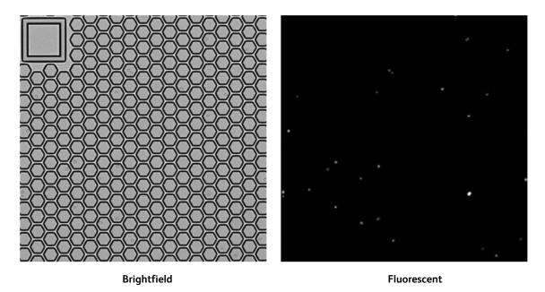
Significant cell loss after the second bead wash: Images after the second bead wash
