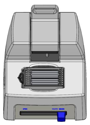
3. Gently pull the top **RETRIEVAL** slider onto the BD Rhapsody<sup>™</sup> 8-Lane Cartridge (ACTIVE). Make sure that the Retrieval magnet is in contact with the BD Rhapsody<sup>™</sup> 8-Lane Cartridge.
