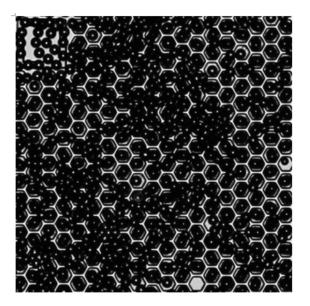
Insufficient loading of BD Rhapsody™ Enhanced Cell Capture Beads after bead loading
