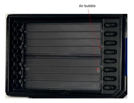
Air bubbles in a cartridge are rare. If there is an air bubble, proceed with the experiment. Follow the user guide to prevent introduction of air bubbles from entering the cartridge.
