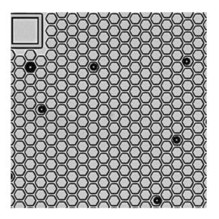
Poor retrieval of BD Rhapsody<sup>™</sup> Enhanced Cell Capture Beads
