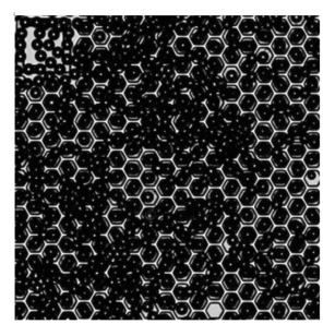
Significant loss of BD Rhapsody™ Enhanced Cell Capture Beads resulting in empty microwells after the second bead wash
