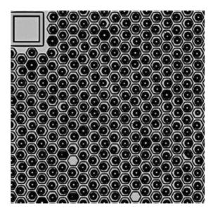
Insufficient removal of excess BD Rhapsody™ Enhanced Cell Capture Beads
