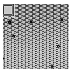
Poor retrieval of BD Rhapsody™ Enhanced Cell Capture Beads
