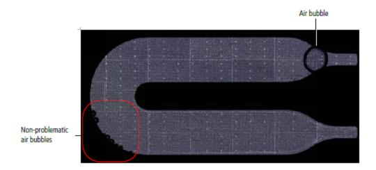
Air bubbles in a cartridge are rare. If there is an air bubble, proceed with the experiment. Follow the user guide to prevent air bubbles from entering the cartridge.
