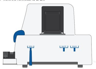
3. Remove the cap of a Waste Collection Container, and insert both the container and a new 5-mL LoBind tube for bead retrieval into the appropriate slots in the drawer. Secure the cap of the 5-mL LoBind tube to the holder:
