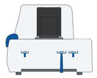
5. Push the cartridge into the far end of the tray to match the cartridge and tray notches. Lay the cartridge flat, and release it. Ensure that the cartridge is flat in the tray and the barcode faces out.
